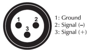
DMX-input XLR mounting-plug:
