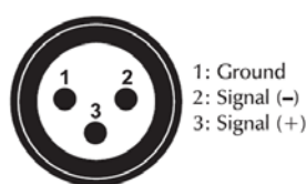
DMX-input XLR mounting-plug:
