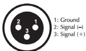
DMX-output XLR mounting-socket:
