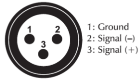
DMX-input XLR mounting-plug:
