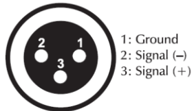
DMX-output XLR mounting-socket:
